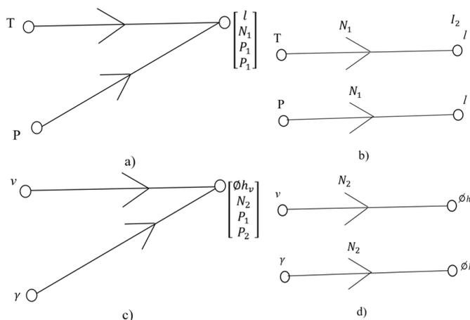
Fig 1. Examples of graph models of FTE: a) model of the effect of thermal expansion; b) model of the Vavilov-Cherenkov effect (radiation); b, d) corresponding single-entry models;  $N_i$  and  $P_j$  – respectively, the number of the FTE and the number of the property.
