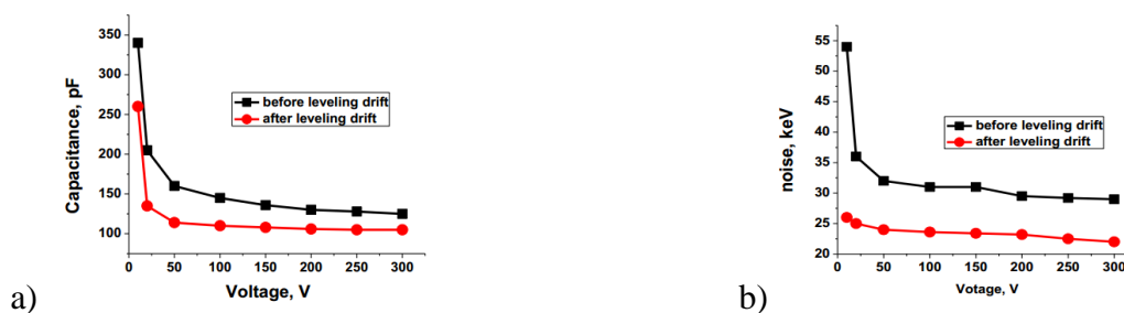
Fig. 1 – Change of the Voltage-Farad and Voltage-Noise characteristics of the detector obtained by Czochralski method with the diameter D = 110 \text{ cm}^2 and thickness W_i = 4 \text{ mm} . Before and after “leveling” drift under temperature T = 65\text{-}70 \text{ }^\circ\text{C} with a reverse bias voltage U_{\text{rev}} = 150\text{-}300 \text{ V} for 15-40 hours
