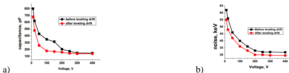
Fig. 2 – Change of the Voltage-Farad and Voltage-Noise characteristics of the detector obtained by float-zone method with the diameter D = 110 \text{ cm}^2 and thickness W_i = 4 \text{ mm} . Before and after “leveling” drift under temperature T = 65\text{-}70 \text{ }^\circ\text{C} with a reverse bias voltage U_{\text{rev}} = 150\text{-}300 \text{ V} for 15-40 hours
