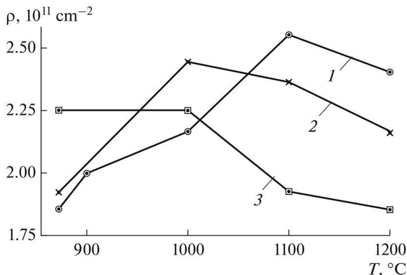
Fig. 2. Influence of the temperature  $T$  on the dislocation density  $\rho$  of quenched steel 45 tempered at 200 °C, when the holding time is 20 min (1), 2 h (2), and 5 h (3).
