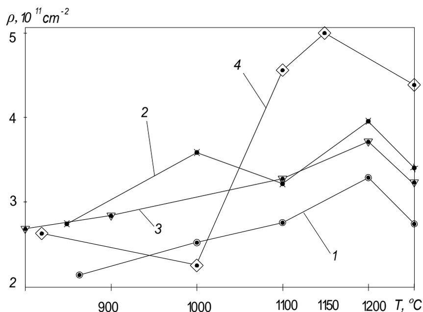
Fig. 3. The density of steel dislocations  $\rho$  after preliminary normalization from various heating  $T$  temperatures. Steel 35 (1); steel 65G (2); steel U8 (3); steel U12A (4).
