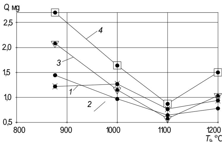
Fig. 4. Dependences of the wear  $Q$  of 40Kh steel under friction with lubrication on the quenching temperature  $T_q$  at the tempering temperature  $T_i = 200$  (1),  $350$  (2),  $450$  (3) and  $600$  °C (4)
