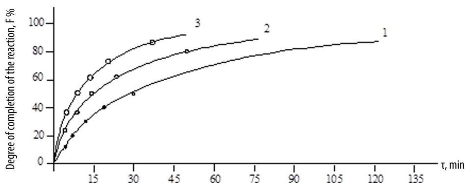
**Figure 3. Degree of completion (F) of polycondensation of CW with furfural from reaction time at different temperatures, catalyst HCl, 5 %. 1-70°C; 2-80°C, 3-90°C.**
