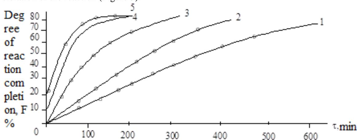
**Figure 5. Degree of completion (F) of polycondensation of furfural with CW over time as a function of catalyst concentration.
