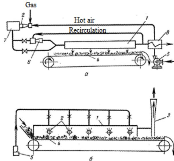
**Fig. 7. Gas-fired thermo-radiation dryers:**
