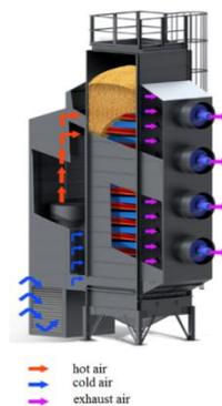
Fig. 2. General view of the mine dryer.
