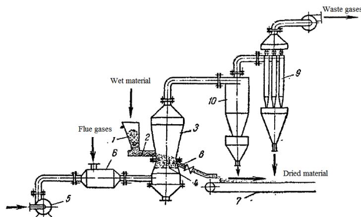
Fig. 4. Single chamber fluid bed dryer.
