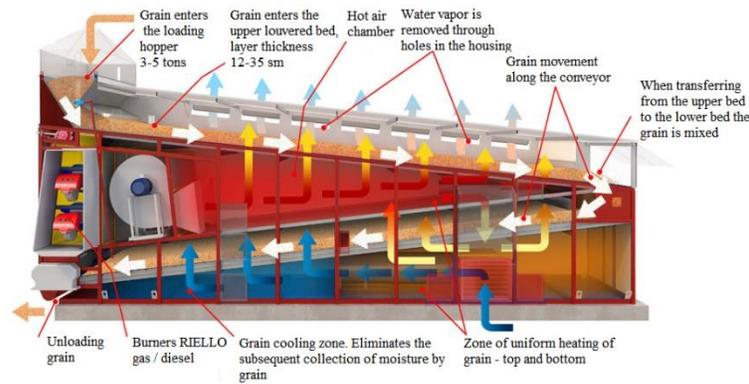
Fig. 3. Conveyor grain dryer diagram.
