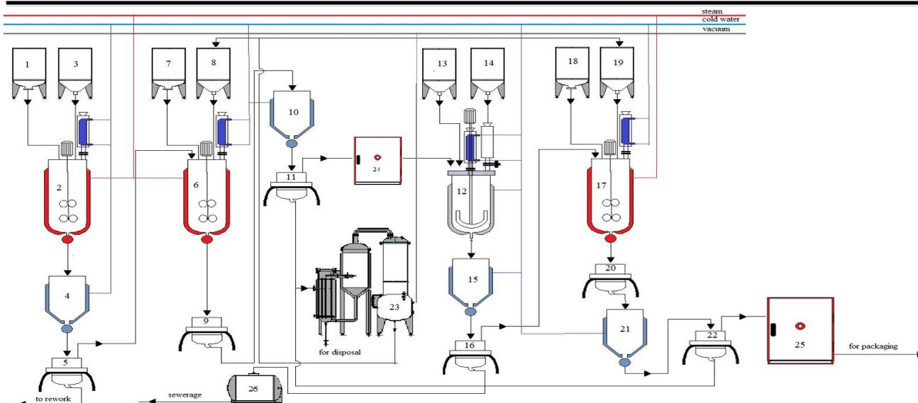
Figure 6. The technological scheme for the production of 5-nitro-2-acetylaminobenzimidazole. 1,7,18-bins; 2,6,17-glass reactors; 3,8,13,14,19-merniks; 4,10,15,21-glass container for cooling; 5,9, 11, 16, 20, 22-filters; 12-glass nitration reactors; 23-vacuum-circulation evaporator; 24,25-oven for drying the finished product; 26-drainage tank.
