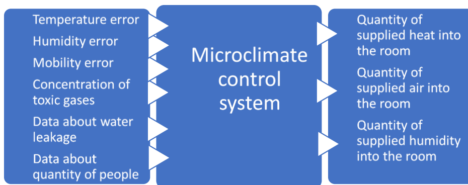
Fig. 3. Generalized structure of the microclimate control system.
