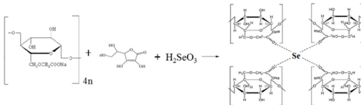
**Fig. 1. Estimated stabilization mechanism and pattern of selenium nanoparticle formation.**
