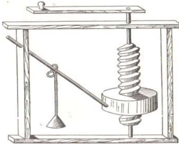
**Figure 7. The appearance of twist-off screw (axis)device**
