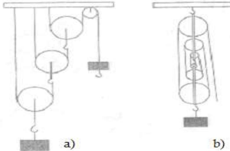
**Figure 4. Different ways of using blocks. a) a device consisting of one fixed block and three movable blocks; b) a system of three blocks mounted on a fixed axis, i.e., three movable and three stationary blocks**
