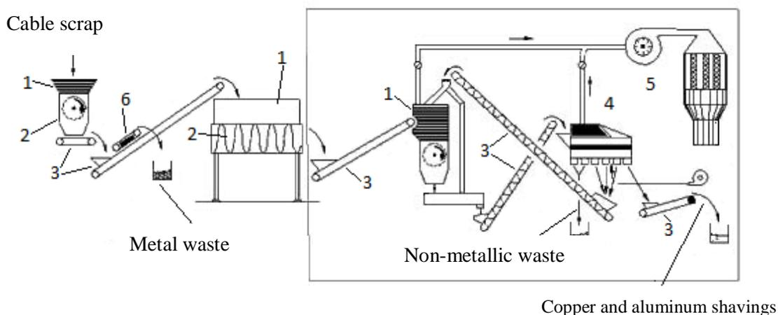
Fig. 2. **Technology line scheme for recycling cable waste:**
