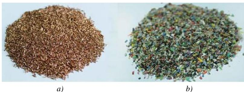
Fig. 1. **Received recyclables:** a) Copper shavings; b) Plastic compound.
