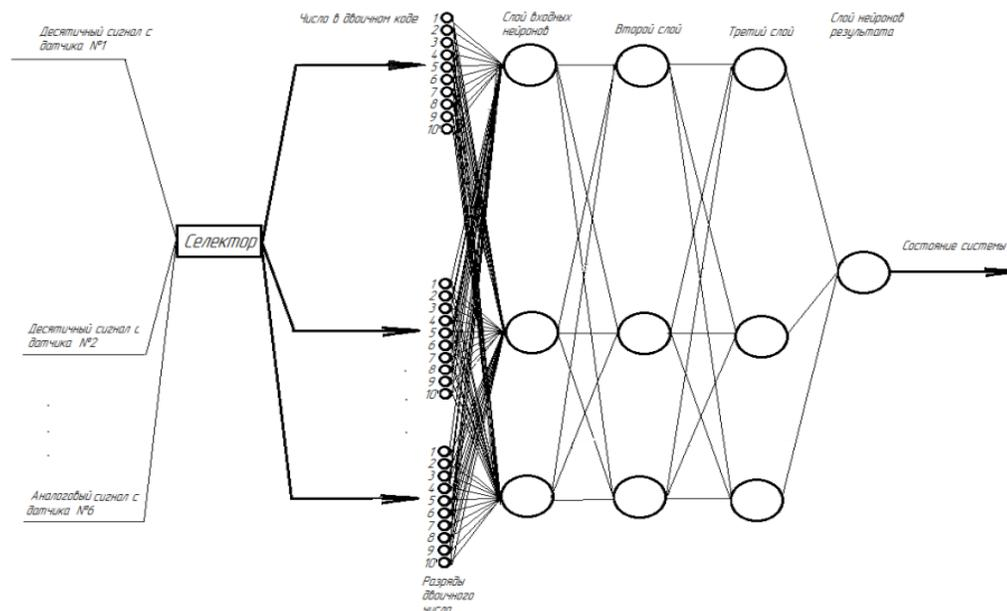
Fig.4. Structure of developed ANN.
