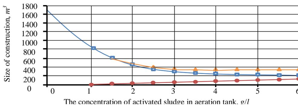
Fig. 3. Volumes of aeration tank and secondary sump and total volume of structures (aeration tank + secondary sump) in high-load processes:
