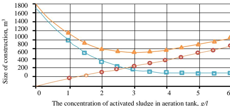
Fig. 2. Volumes of aeration tank and secondary sump and total volume of structures (aeration tank + secondary sump) in high-load processes:
