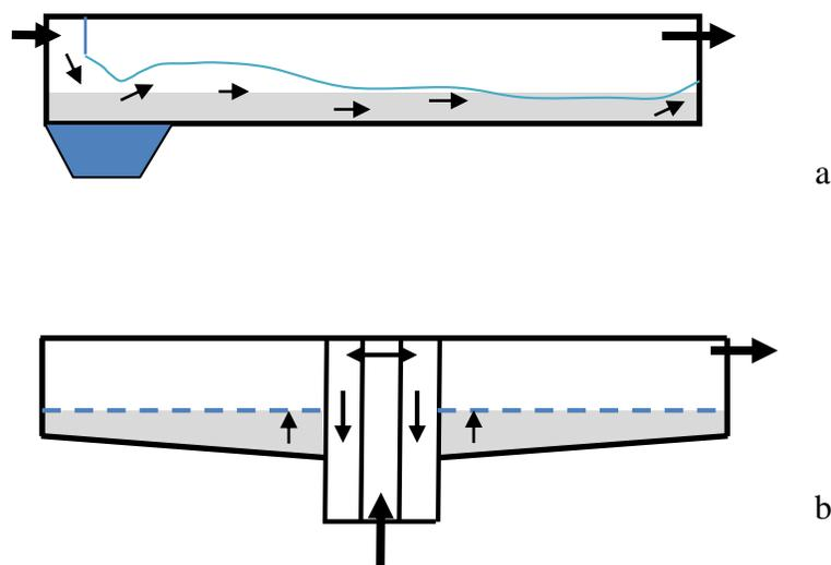
Figure 1. Schematic flows in a rectangular (a) and radial (b) secondary sedimentation tanks.
