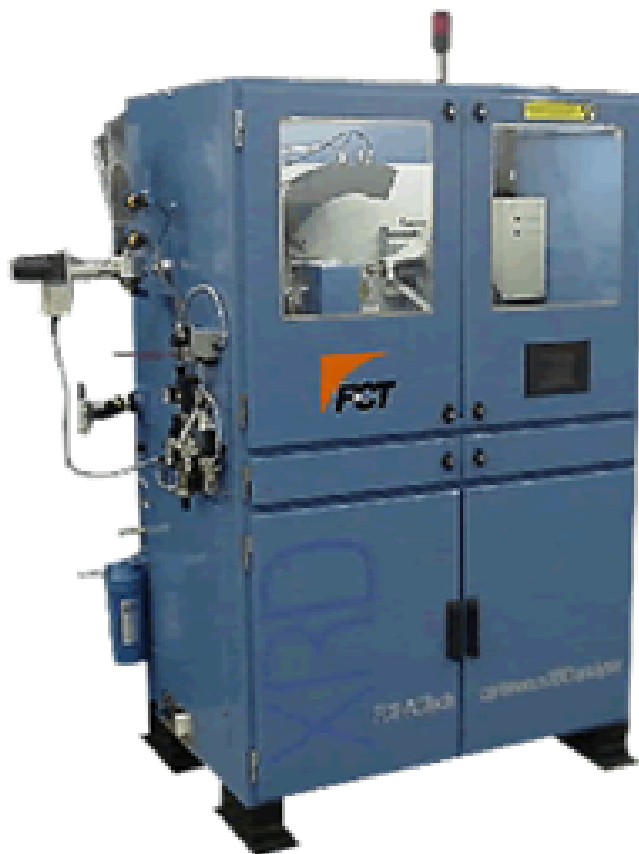
Fig. 1: Mineralogical and phase analysis diffractometer - COSMA.
