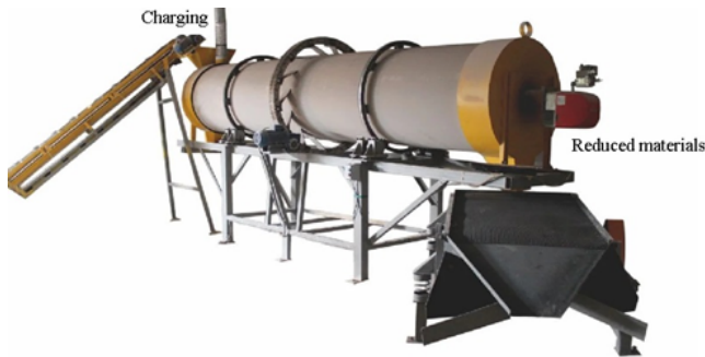
Fig. 5: Rotary tube furnace (Waelz furnace).
