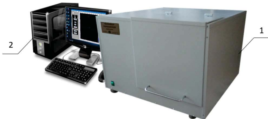
Fig.2. General view of the SCAN-2019 installation: 1 - measuring system SCAN-2019; 2 - personal computer
