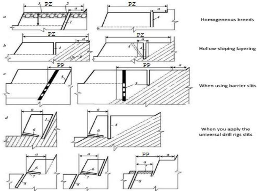
**Fig. 1.** Diagrams of the location of protective slits in the contact zone (PZ):
