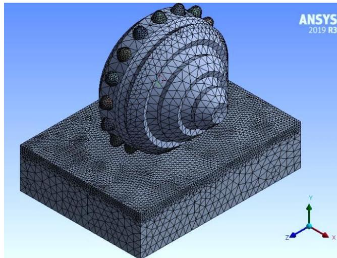
**Fig.3.** Mesh Settings of the cone and rock
