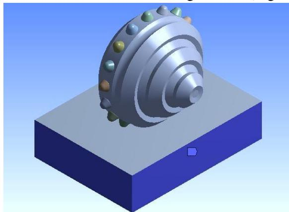
**Fig. 4.** Model with fixed rock sides
