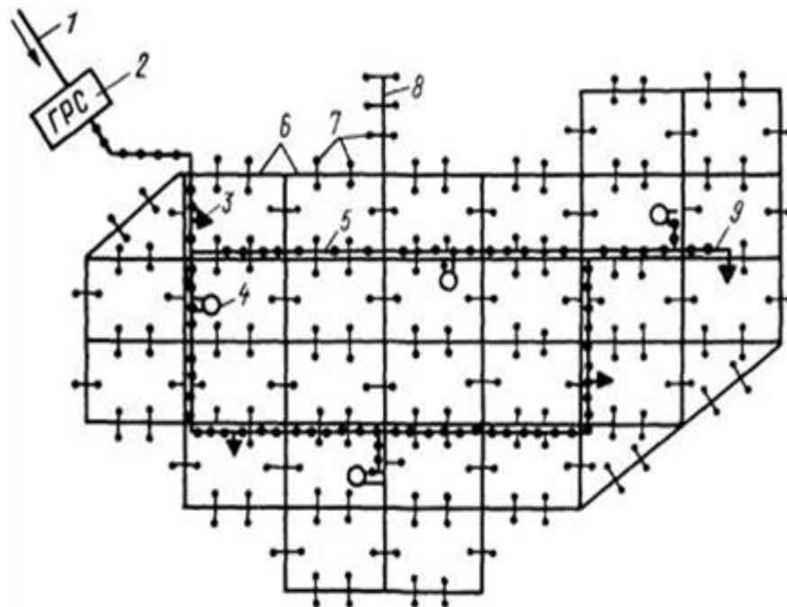
**Figure 3.** - Diagram of a two-stage gas distribution system. 1 - high pressure main gas pipeline; 2 - GRS; 3 - large gas consumers; 4 - city hydraulic fracturing stations supplying low pressure gas pipelines; 5 - high and medium pressure gas pipelines; 6 - ring low pressure gas pipelines; 7 - branches to consumers; 8-9 - dead-end gas pipelines (8 - low pressure, 9 - medium pressure).
