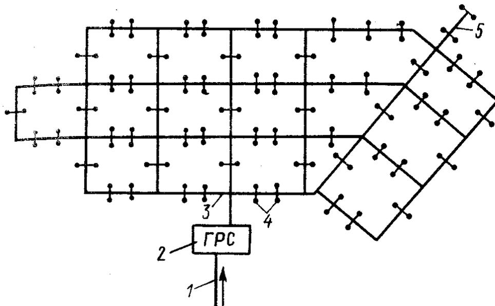
**Figure 2.** Diagram of a one-stage gas distribution system. 1 - main gas pipeline; 2 - GRS; 3 - ring gas pipelines; 4 - branches to consumers; 5 - dead-end gas pipelines.
