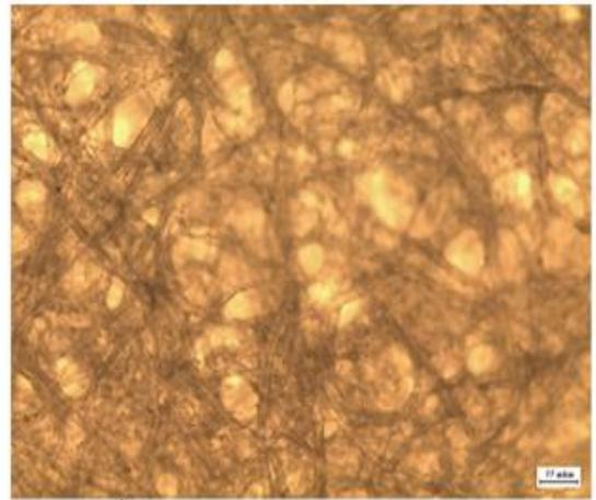
**Microphotographs of the surface of paper made from 90% CC: 10% MC**
