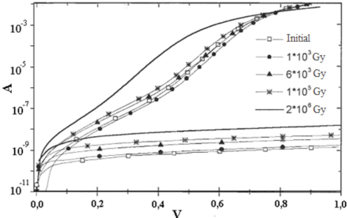
*Fig.1. Forward and reverse branches of the V-A characteristic by a diode with Schottky barriers Au-GaAs from a moth-eye interface: initial and irradiated with  $^{60}\text{Co}$  gamma quanta to doses of  $10^3$ ,  $6 \times 10^3$ ,  $10^5$ ,  $2 \times 10^6$  Gy, respectively*
