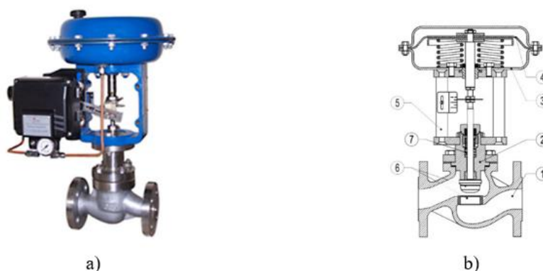
Fig. 1. Diaphragm pneumatic control valve: a) photo of the valve; b) valve drawing; 1) output channel; 2) valve body; 3) inlet channel controlling pressure; 4) membrane; 5) drive; 6) a saddle and a lock; 7) stock
