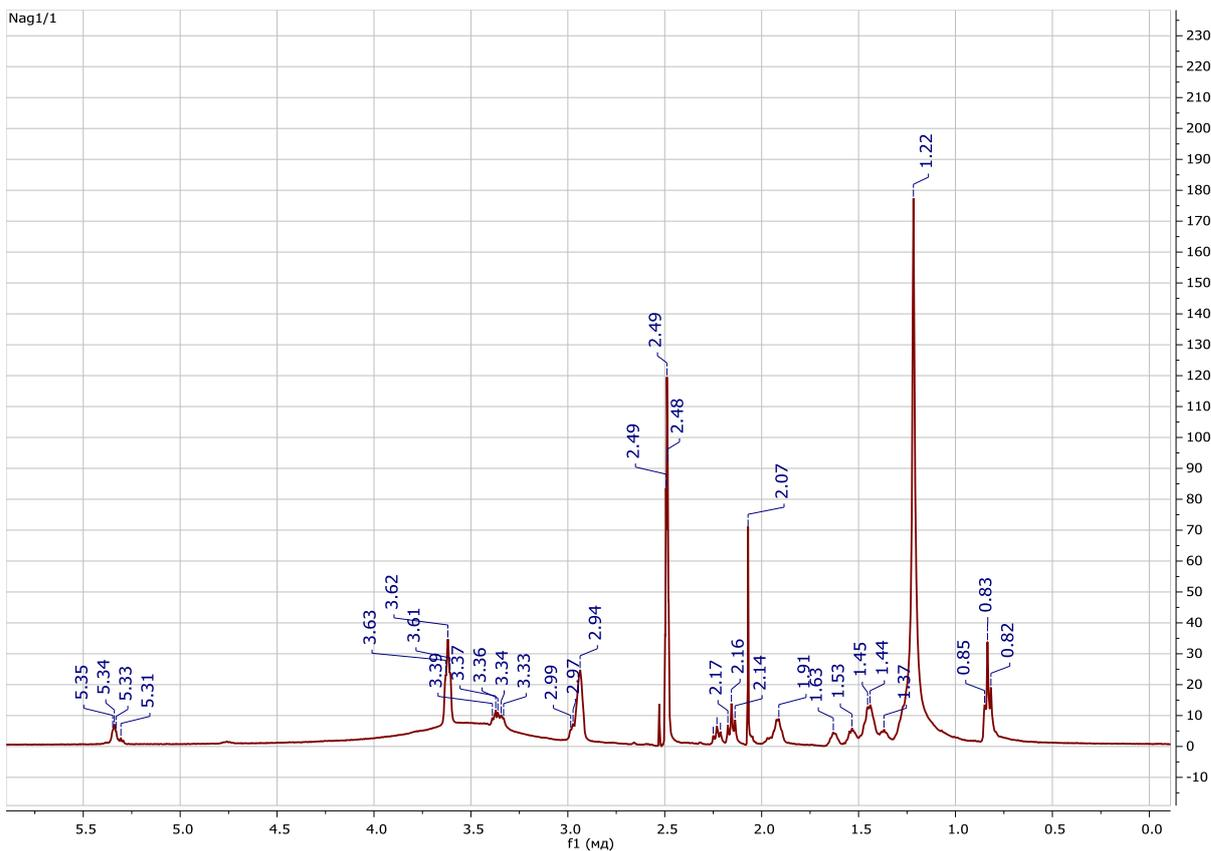
**Figure 2.** NMR, <sup>1</sup>H spectrum of salts of sulfated oleic acid amides based on piperidine.
