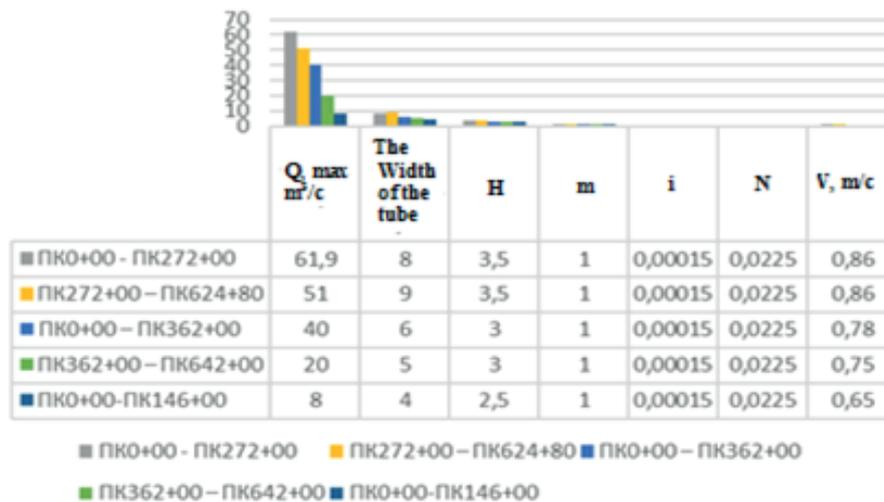
Figure 3. Quantitative indicators of reliable operation of sections of the Greater Namangan Canal.
