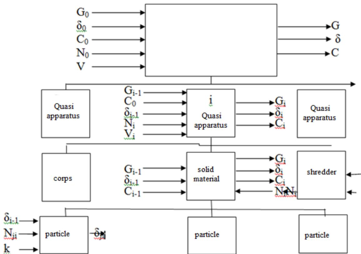
The object being investigated - the jaw crusher is taken as a primary large technological system (first hierarchical level). In it the cumulative process takes place. Indicators are determined - input, output parameters of the object - system and the process occurring in the system.
