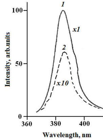
**Figure 3:** the PL spectra of nanopowders (1) and micropowders ZnO, obtained at room temperature.
