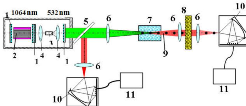
*Figure 1: schematic diagram of an experimental setup for the study of powders. 1 – laser mirrors, 2 – active medium – YAG:Nd<sup>3+</sup>, 3 – nonlinear crystal, 4, 6 – lenses, 5 – quartz plate, 7 – cuvette, 8 – photonic crystal, 9 – secondary radiation, 10 – minispectrometr, 11 – computer.*
