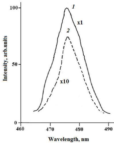
**Figure 2:** the PL spectra of nanopowders (1) and micropowders ZnSe, obtained at room temperature.
