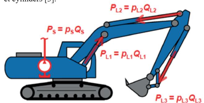
Figure 1. Mobile excavator with indication of powers [3]
