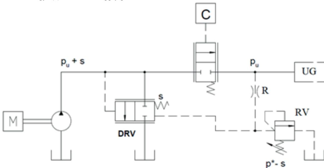
Figure 2. Load sensing plant with constant displacement pump [4]
