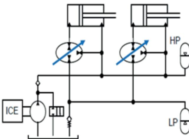
Figure 7. Constant pressure system with hydraulic transformers
