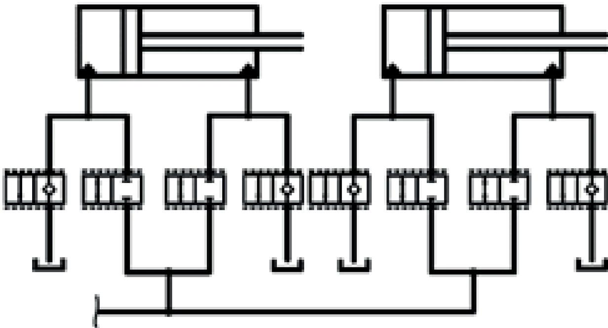
Figure 5. Digital flow control ISO scheme.
