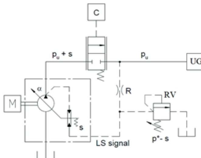
Figure 3. Configuration with differential pressure variable displacement pump [4].
