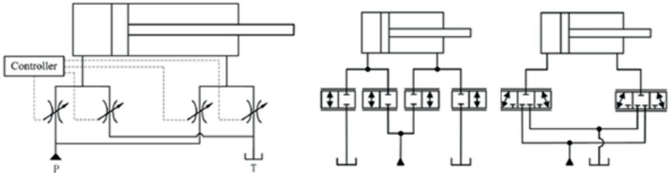
Figure 4. Possible layouts of independent metering.
