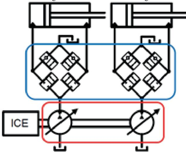
Figure 6. Displacement control with independent metering.
