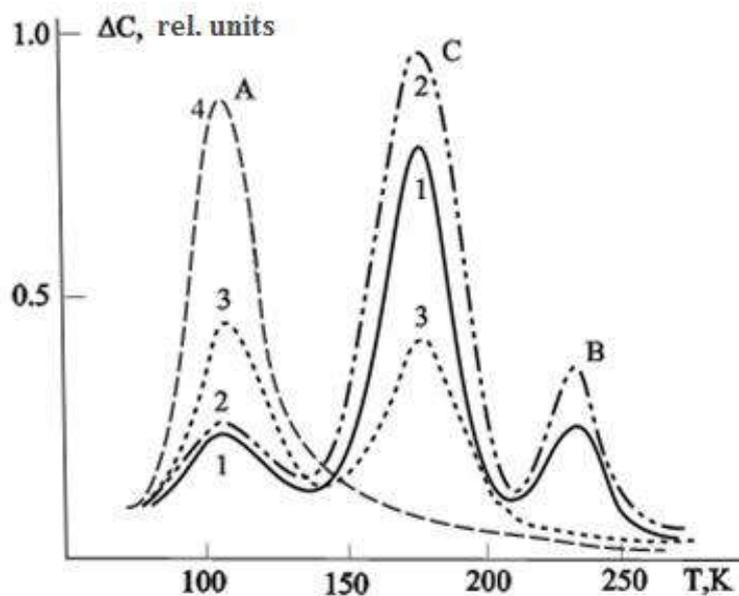
**Fig. 2. DLTS spectra of  $n\text{-Si} \langle \text{Mn} \rangle$  samples with bonded oxygen states**
