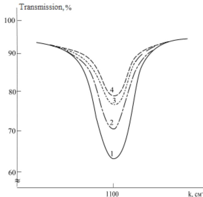
**Fig. 1 Typical infrared absorption spectra of control samples *n*-Si (curve 1), *n*-Si <Mn> (curve 2), *n*-Si + heat treatment (curve 3), *n*-Si <Mn> with preliminary heat treatment at 1100°C (curve 4).**
