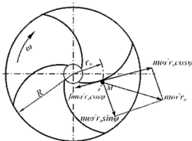
Figure 1.  $r_0$  scheme of distance determination
