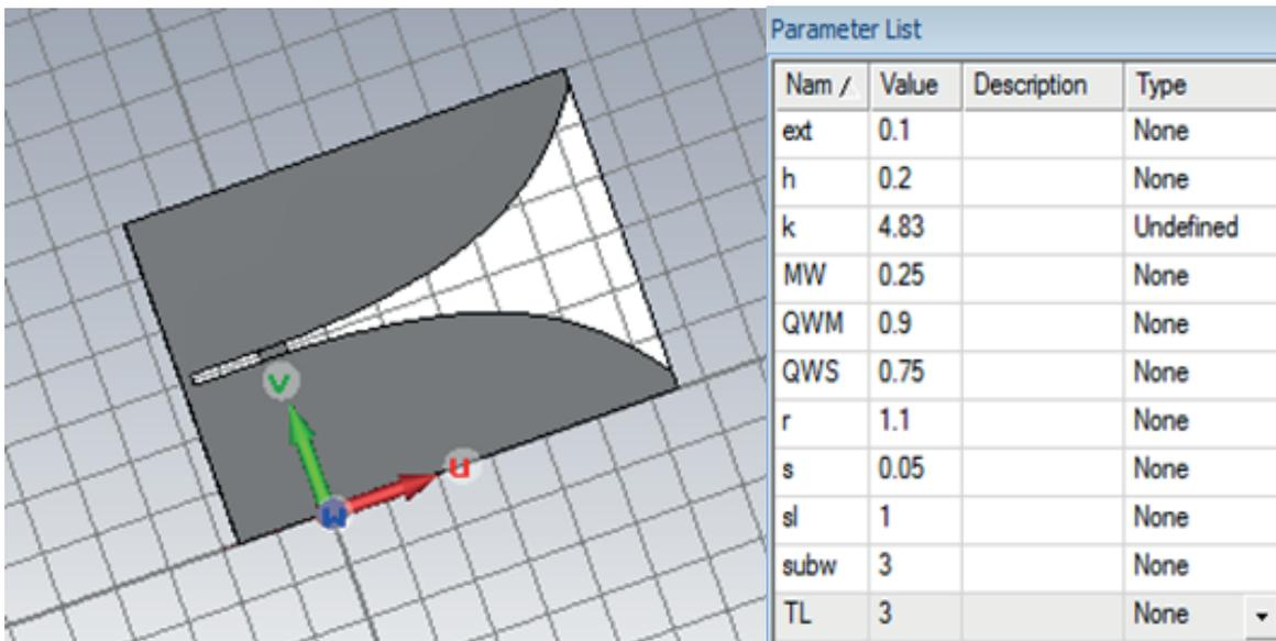
Fig. 2. The physical model of the antenna made in CST.
