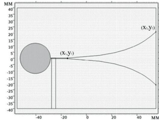
**Fig. 1. The geometric dimensions of the antenna**
