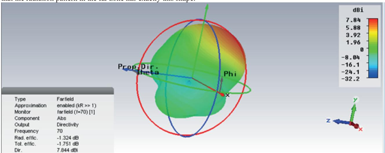
Fig. 3. 3D pattern of the Vivaldi antenna at 70 GHz.
