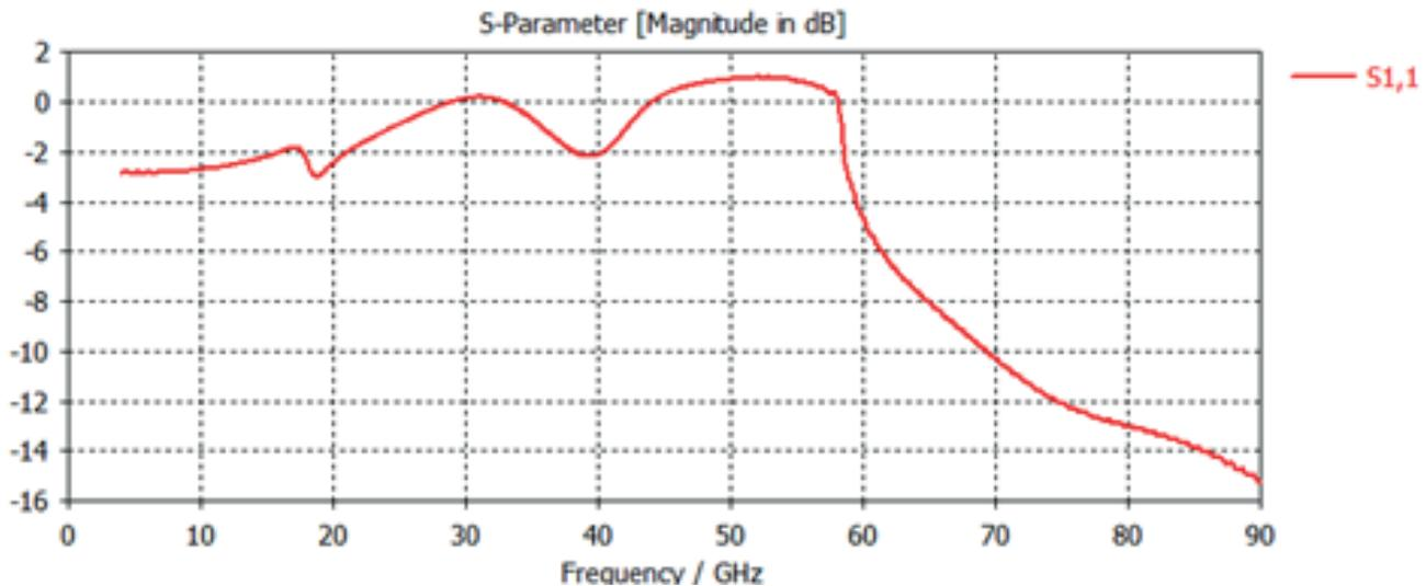
Fig. 4. The return loss of the Vivaldi antenna at 70 GHz.
