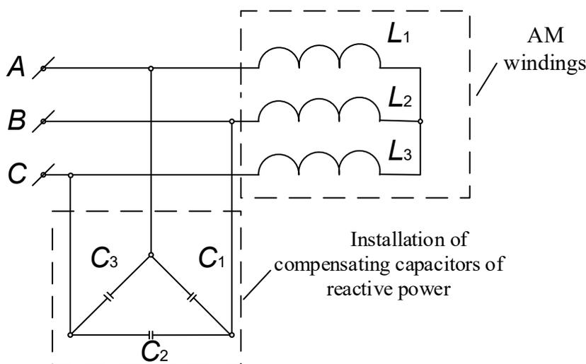
**Figure 2 - Diagram of the connection of compensating capacitors  $C_1, C_2, C_3$  to the AM windings.**
