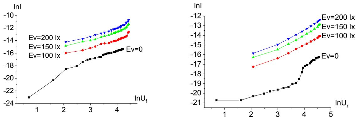
**Fig. 2.** Volt-ampere characteristics of  $\text{Au-nAl}_{0.1}\text{Ga}_{0.9}\text{As-pGaAs-Ag}$ -structure in double logarithmic scale in the mode of (a) direct and (b) reverse bias of the heterojunction
