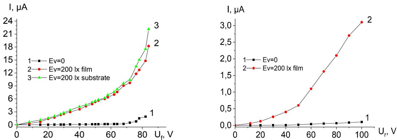
**Fig. 1.** Volt-ampere characteristics of the  $\text{Au-nAl}_{0.1}\text{Ga}_{0.9}\text{As-pGaAs-Ag}$  structure in the mode of (a) direct and (b) reverse bias of the heterojunction
