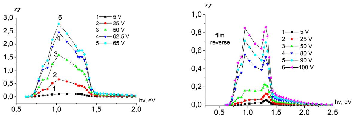
**Fig. 3.** Spectral sensitivities with illumination from the side of a reverse biased heterojunction (a) and from the side of a forward biased heterojunction (b)
