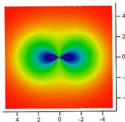
**Figure 4:** The calculated dependence of the phase difference shift in a crystal with a symmetry of 3 m, due to a change in the refractive index, depending on the intensity of laser radiation
