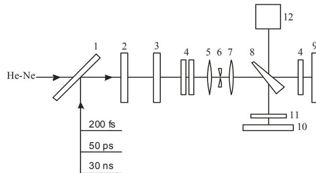
**Figure 1: Scheme for recording phase holograms. 1 mirror. 2,3 - nonlinear frequency multiplication crystals. 4- light filters. 5,7- lens. 6 -spatial filter. 8 -optical wedge. 9-10 - mirror. 11 - test sample. 12- CCD camera.**
