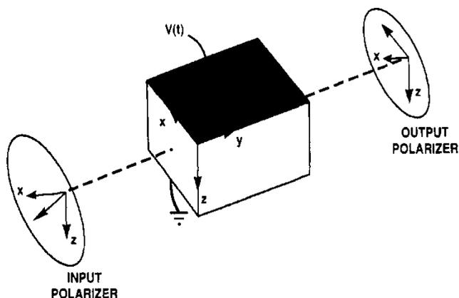
Figure 4. Bulk electrooptic intensity modulator consisting of an input polarizer oriented 45° with respect to the modulator axes, a polarization-dependent electrooptic phase modulator, and an output polarizer oriented 90° with respect to the input polarizer.
