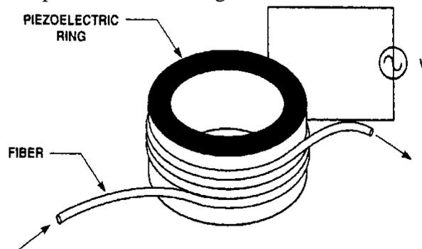
Figure 7. Fiber optic phase modulator consisting of a fiber coiled around a piezoelectric ring. Application of voltage changes the ring diameter and the fiber length.
