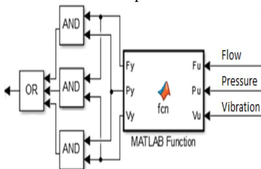
Fig 3. The structure of the element of majority voting
