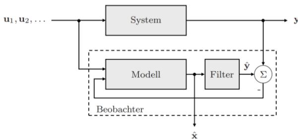
Fig. 1 Block diagram of the virtual analyser.
