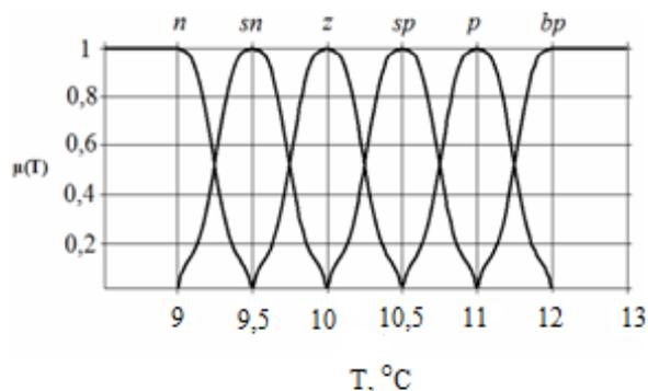
Fig. 3. The membership functions of the value "Temperature in the storage" to the terms of the linguistic variable "Temperature mode"
