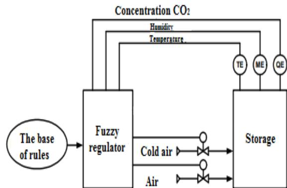
*Fig. 1. Schematic diagram of the automation of the process control system of storage of perishable oilseeds.*
