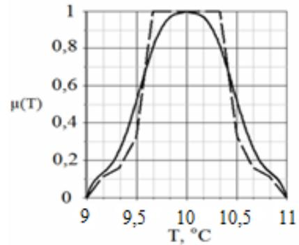
Fig. 2. The membership function for the term "sn": dotted line - piecewise linear characteristic; solid line - approximation by Lagrange polynomials.
