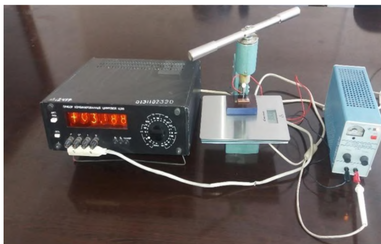
Fig. 2. Appearance of the installation for measuring the parameters of samples under the influence of external pressure
