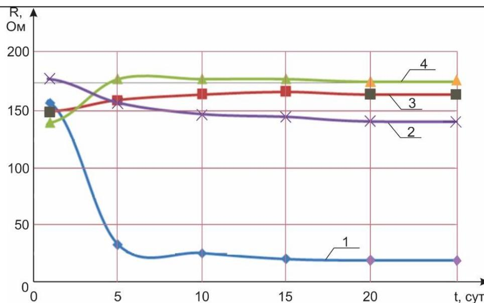
**Fig. 2.** The dependence of the polarization resistance from time to time in 98% H<sub>2</sub>SO<sub>4</sub> solution 1 - uncoated; 2 - OMKM3; 3 - OMKM1; 4 –OMKM2.
