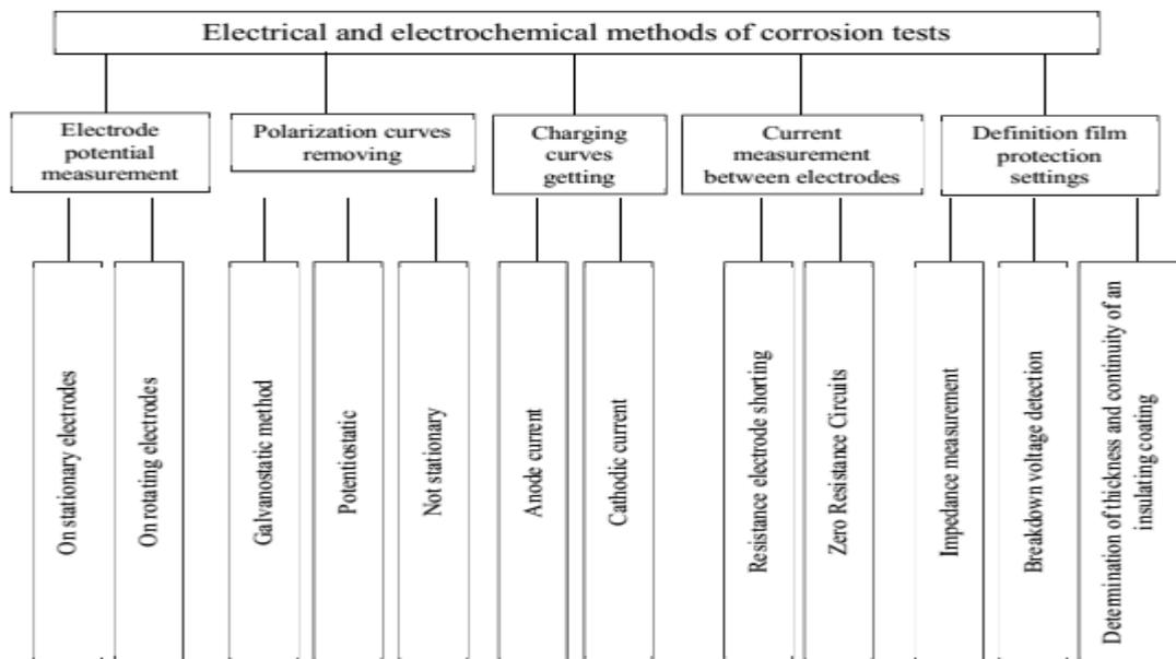
**Fig 1.** Corrosion test methods based on measuring electrical quantities.
