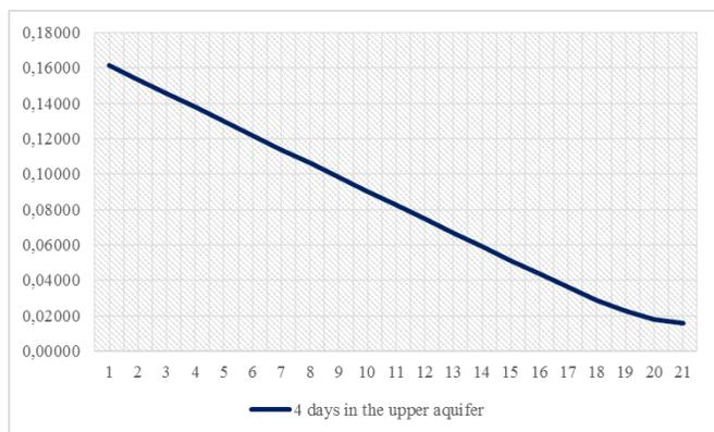
Figure 2: Changes in pressure in the upper filtration layer without taking into account the elastic regime.
