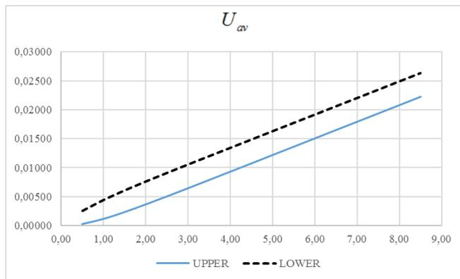
Figure 9: Average overflow rate in the upper and lower aquifers
