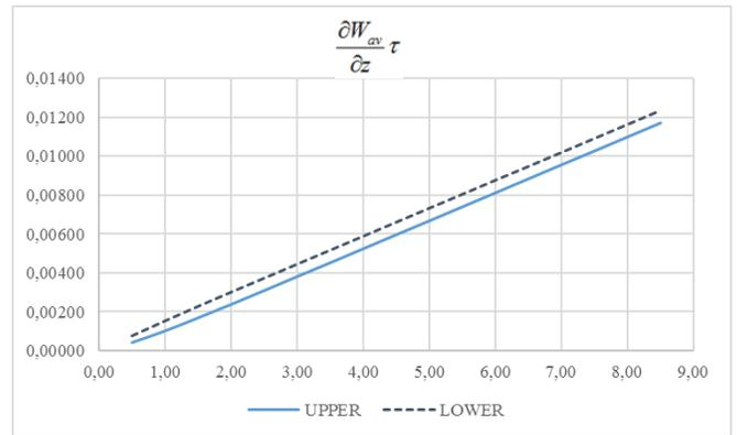
Figure 7: Average change in the gradient of the filtration rate in the upper and lower aquifers
