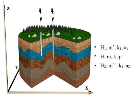
**Figure 1:** Schematic representation of a three-layer area of filtration
