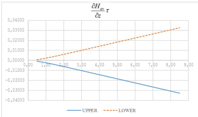
Figure 4: Average change in pressure gradient in the upper and lower aquifers
