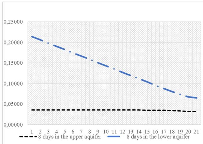
Figure 1: Changes in pressure in the layers along the length of filtration layers without taking into account the elastic regime.
