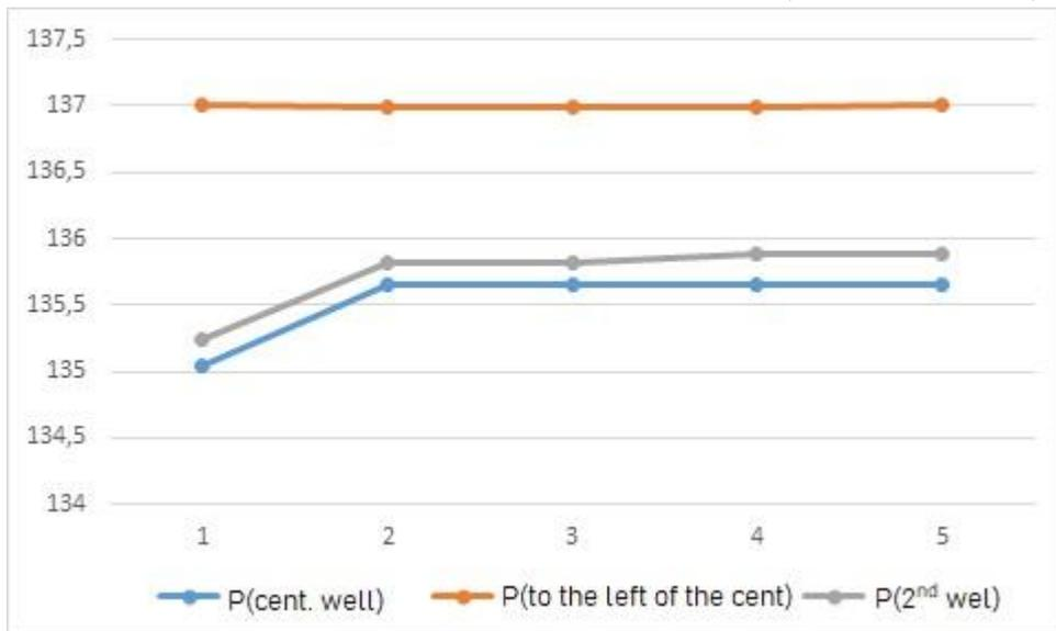
Fig. 5. Change in gas pressure in wells and in neighboring corners (at  $t=49580.233 h$ )
