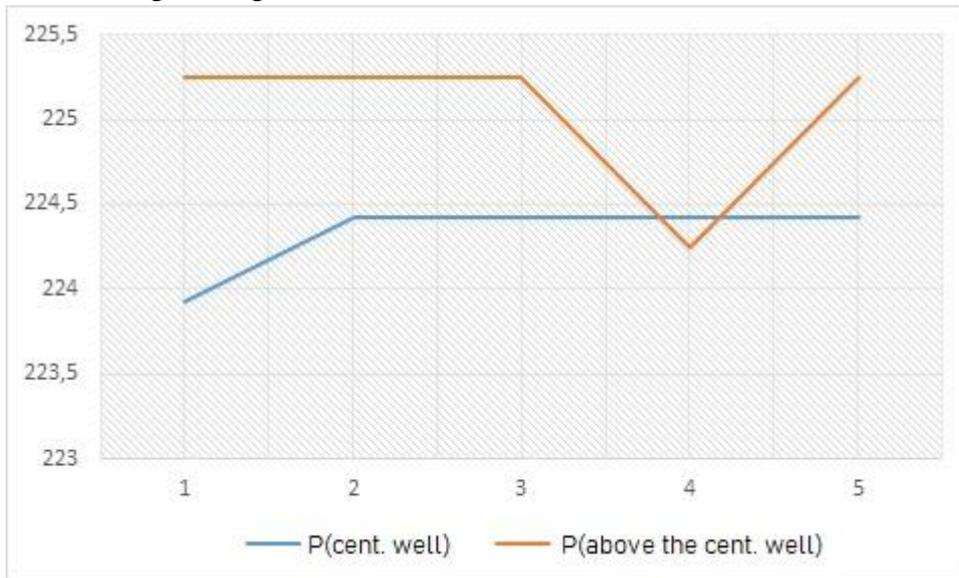
Fig. 3. Change in gas pressure in wells and in neighboring corners
