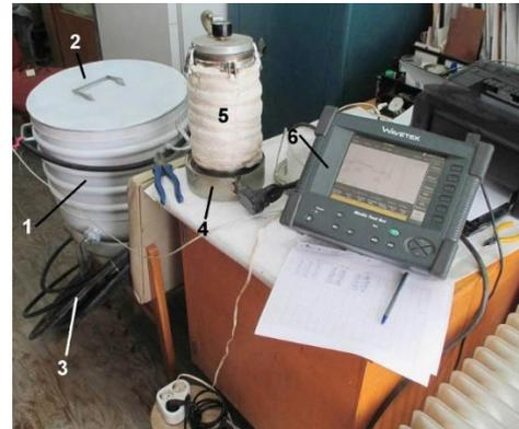
Fig.6. Photo of an experimental complex for studying the optical parameters of a fiber-optic cable with a change in temperature:
