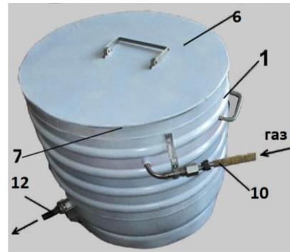
Fig.4. External view of the climatic chamber: 1 - the outer casing of the climatic chamber; 6 – cover of the outer casing of the climatic chamber; 7-layer special insulator of the climate chamber cover; 10 - thermally insulated tube; 12 - outlet branch pipe
