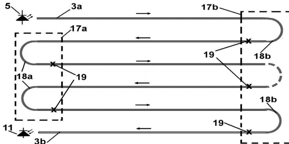
Fig.7. Schematic diagram of switching single-mode optical fibers of a multicore optical cable: 3a - lead-in end of the fiber-optic fiber; 3b - Lead-out end of optical fiber; 5 - emitting laser; 17a - external cassette; 17b - inner cassette; 18a, b - loops of optical fiber with splice points; 19 - optical fiber splice points
