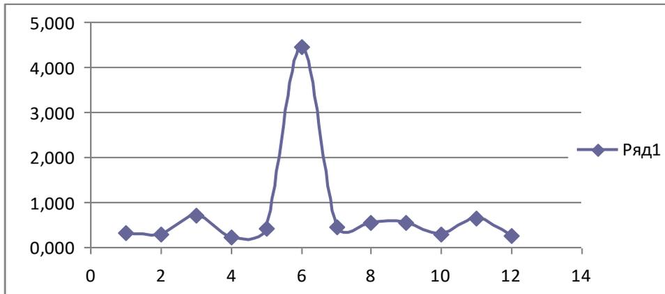
Fig.8. The graph of the attenuation dependence for twelve investigated sections of the OF at a temperature of + 18°C
