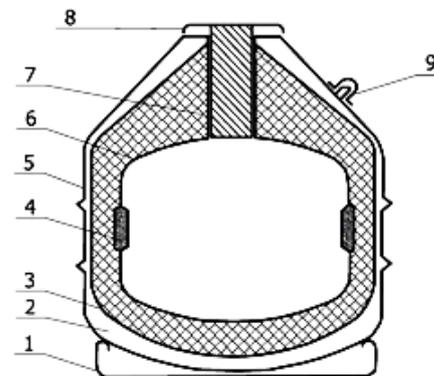
Fig.2. Dewar vessel diagram:
