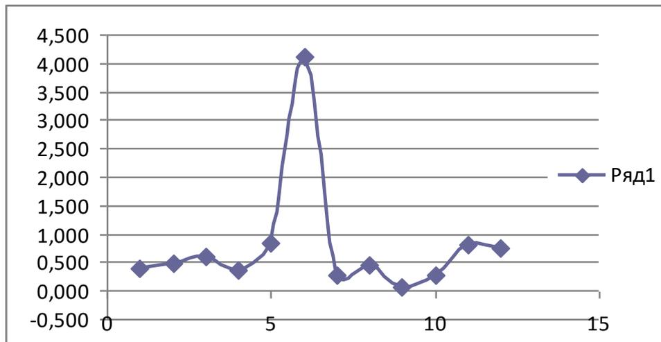
Fig.9. The graph of the attenuation dependence for twelve investigated sections of the OM at a temperature of + 35°C (temperature rise)
