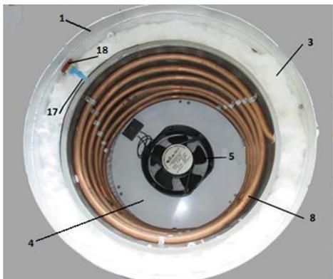
Fig.3. Internal view of the climatic chamber (top view): 1 - external casing of the climatic chamber; 3- mineral wool; 4- bottom of the inner case of the climatic chamber; 5-fan; 8 - copper coil; 17 - electric multicore cable; 18 - electrical connector
