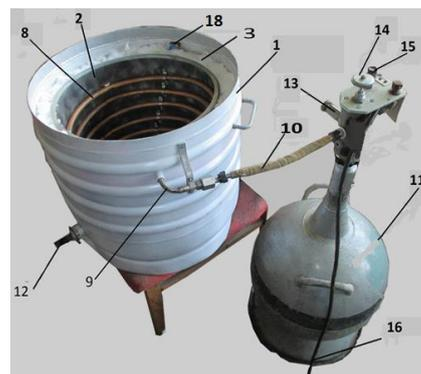
Fig.5. General view of the climatic unit: 1 - the outer casing of the climatic chamber; 2 –inner body of the climatic chamber; 3 - thermal insulating mineral wool; 8 - copper coil; 10- thermally insulated tube; 11 - Dewar vessel; 12 - outlet branch pipe; 13, 14 - taps for supply and regulation of liquid nitrogen; 15 - handle of a variable resistor for regulating nitrogen evaporation; 16 - electric cable; 18 - electrical connector
