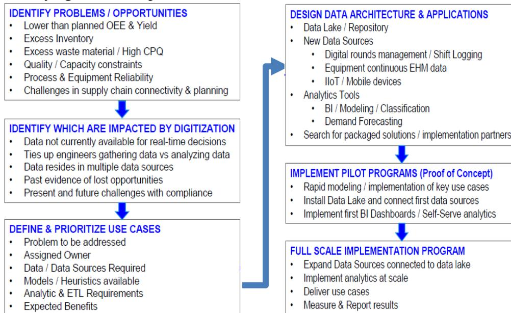
Figure 5. Digitization methodology from Honeywell Connected Plant
