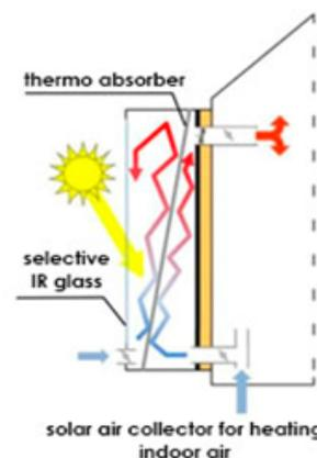
Fig. 4. SAC with heat recuperator
