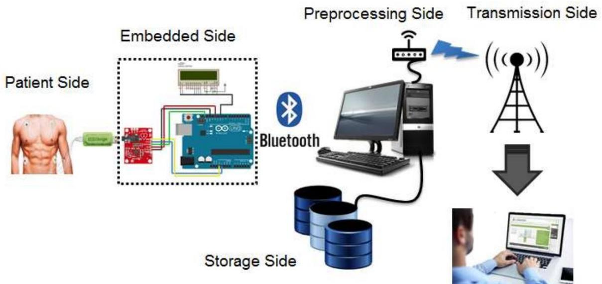
Figure 1. Overall ECG Signal Surveillance System Infrastructure
