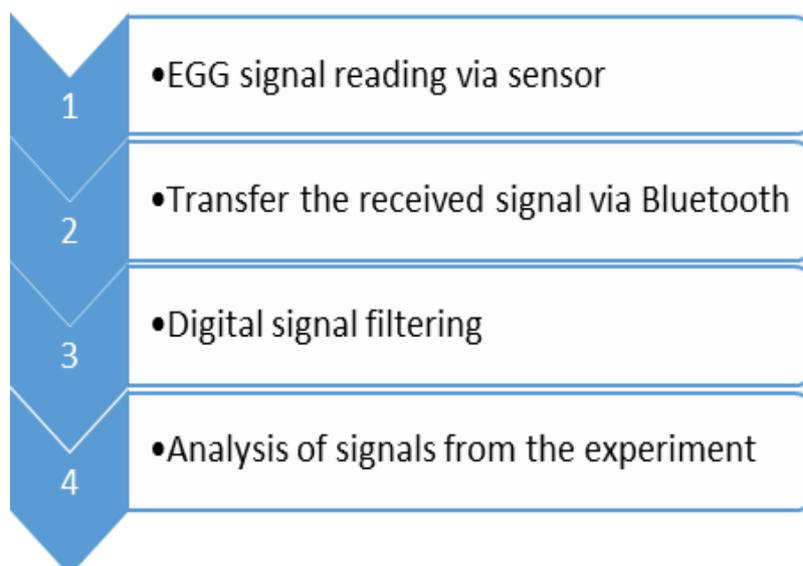
Figure 2. Stages of the process of implementing an EGG signal received from a patient using IoT technology.
