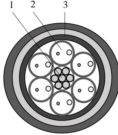
Figure 7. Example of a spiral arrangement of an optical module in FOC: 1-reinforcing elements; 2-optical module; 3-shell FOC
