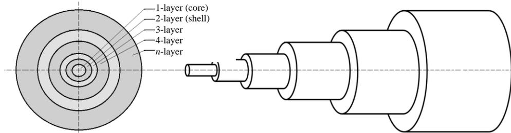
Figure 1. Generalized block diagram of a fiber-optic cable
