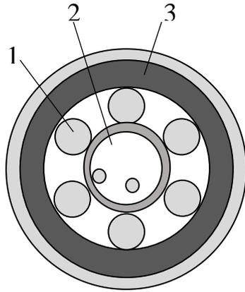
Figure 6. Example of a straight-line arrangement of the optical module in the FOC: 1-reinforcing elements; 2-optical module; 3-shell FOC
