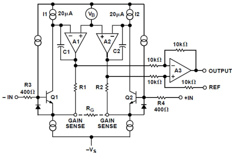
Figure 2. Simplified schematic of AD620
