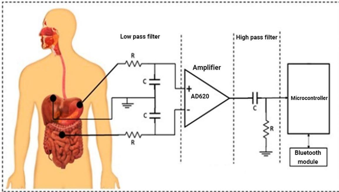
Figure 1. Circuit diagram of EGG measuring device
