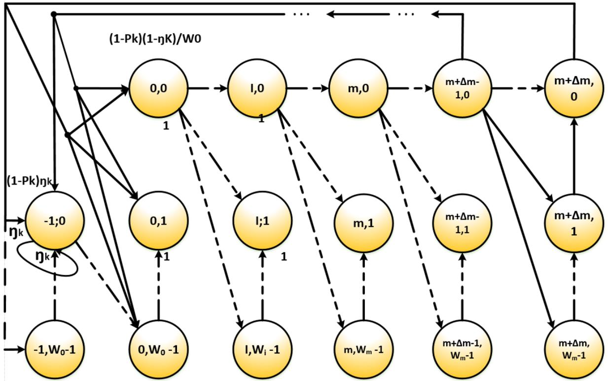
Figure 2. Markov chain describing the assessment of the status of network stations based on the ZigBee standard for monitoring systems.
