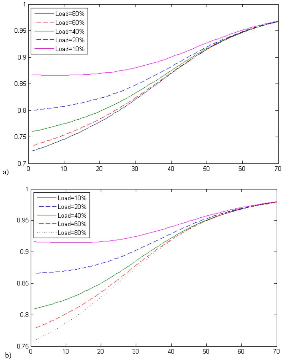
Figure 5. Graph of the dependence of the probability of successful transmission of packets on the number of nodes: a)  $P_f = 0.1$ ; b)  $P_f = 0$ .
