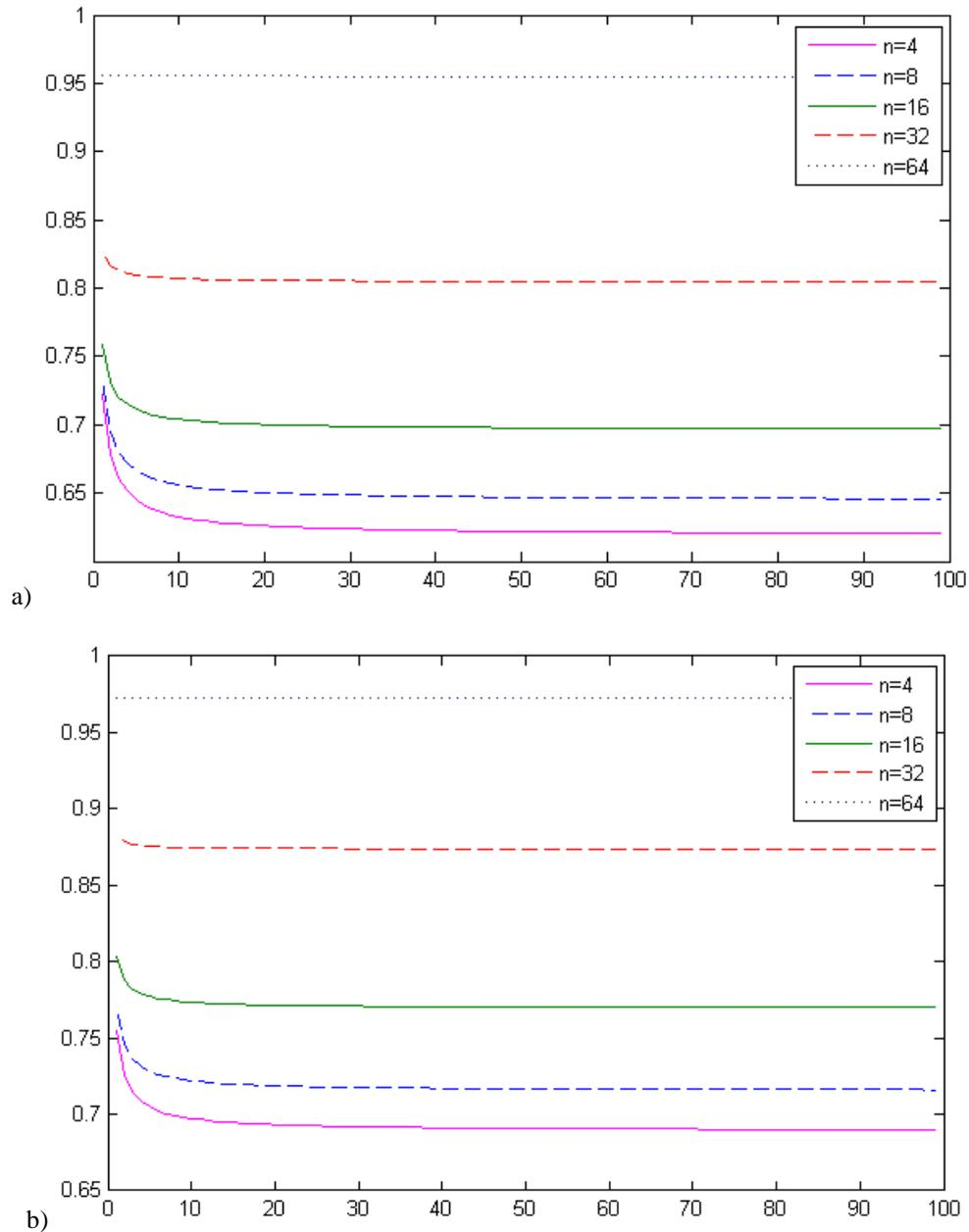
Figure 3. Graph of the dependence of the probability of successful transmission of packets on the system load: a)  $P_f = 0.1$ ; b)  $P_f = 0$ .
