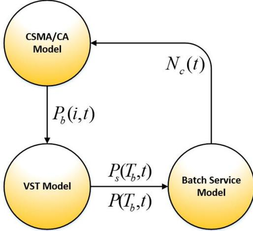
Figure 1. Submodels of the operation process of the wireless sensor network based on the ZigBee standard for monitoring systems.
