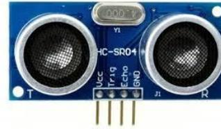
Fig. 7. Ultrasonic sensors
