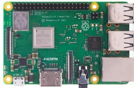
Fig. 8. Raspberry Pi 3 Model B+
