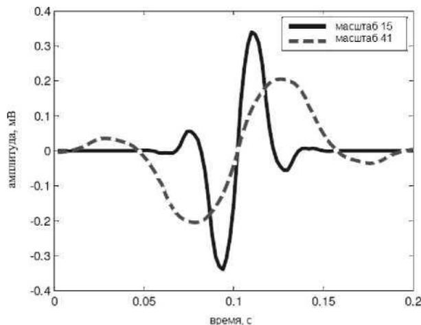
Figure 1. The bior 1.5 wavelet at scales 15 and 41
